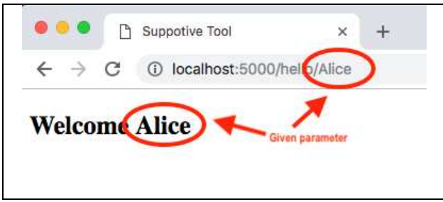
Fig. 7 Response from the WSGI server with parameter
