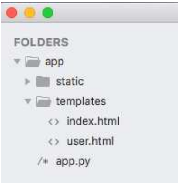
Fig. 3 MVC Model Directory on Flask Microframework
