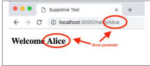
Fig. 7 Response from the WSGI server with parameter
