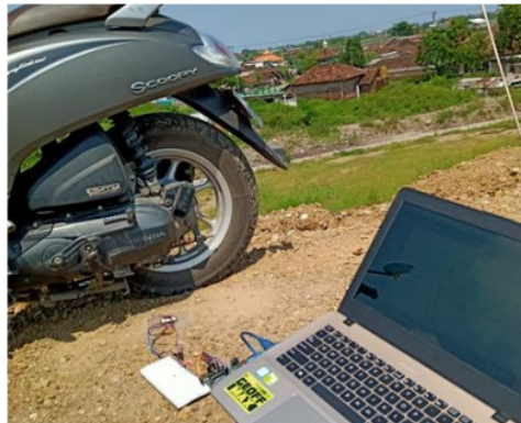
Figure 14. Accelerometer Testing at the Lapindo Embankment
