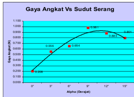
Figure 3. Graph of the amount of lift against the angle of attack.
