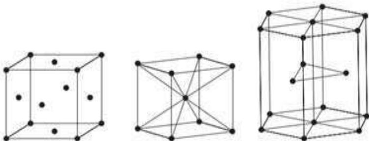
Gambar 4.2 The three most common crystal structure in metals and alloys. Left: face centred cubic (FCC) Centre: Body centred cubic (BCC) and right: hexagonal close packed (HCP). Source: Md. Ibrahim Khan, Welding Science and Technology
