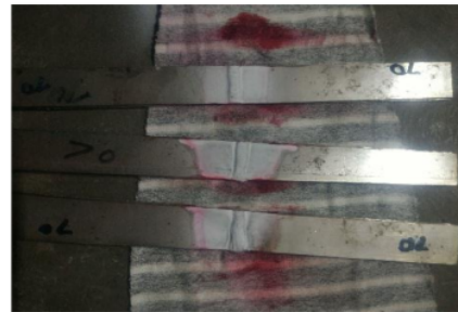
Fig. 3. Dye penetrant test.
