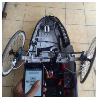
Figure 12. Electric car steering system and application Boarduino
