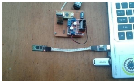
Figure 5. Testing Bluetooth HC 05
