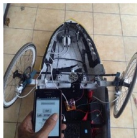
Figure 12. Electric car steering system and application Boarduino
