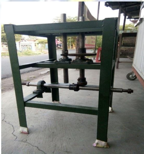
Proses Assembly Transmisi
