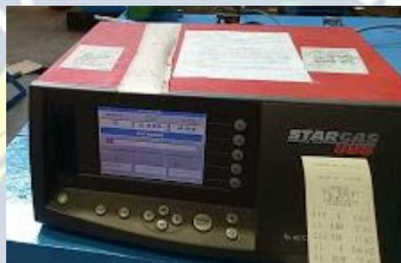
Gambar 3.12 Automotive Emission Analyzer Stargas 898
