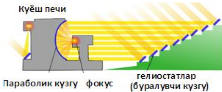
Figure 2. Structure of a large solar oven.
