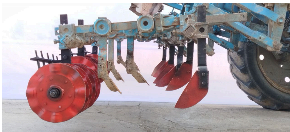
Figure 4. Working body with a razor blade and disk, which is installed on the KXU-4 cultivator.
