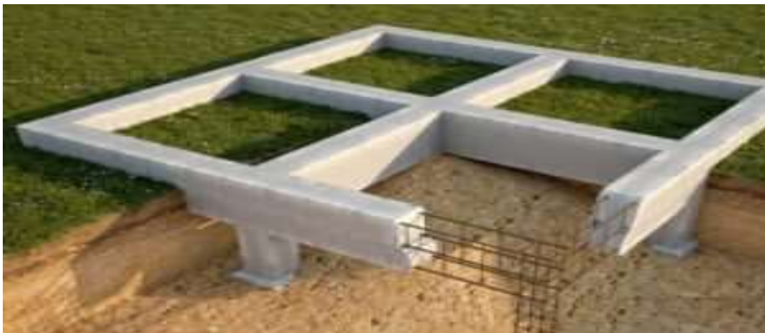
1.2-image. Pile foundation installed on loamy soils
