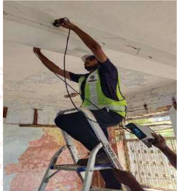
Ultrasonic Pulse Velocity Test
