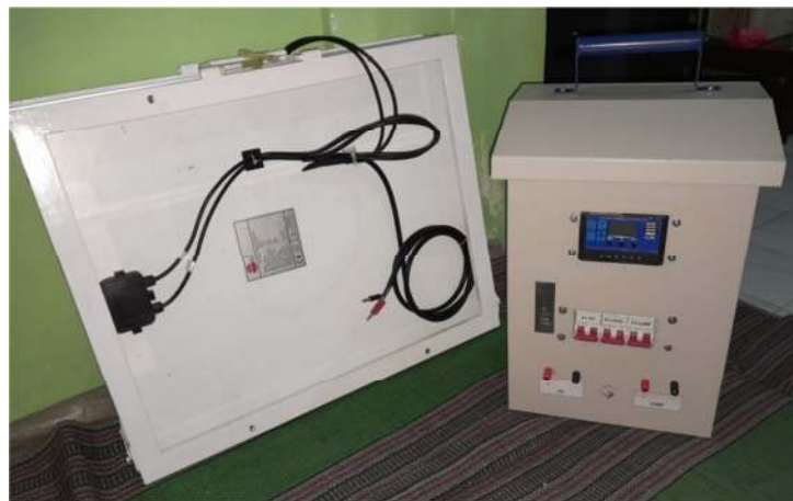
Gambar 2.1. Panel Photovoltaic dan Box Control
