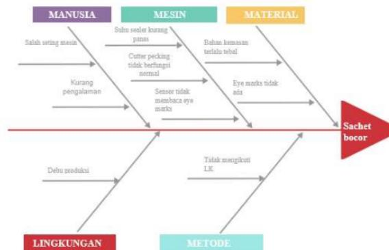
**Gambar 7.** Fishbone diagram sachet bocor
