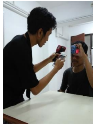
Figure 3. Testing the accuracy of body temperature sensors (MLX90614) against temperature measuring devices (Infrared Thermometer (IR60)).
