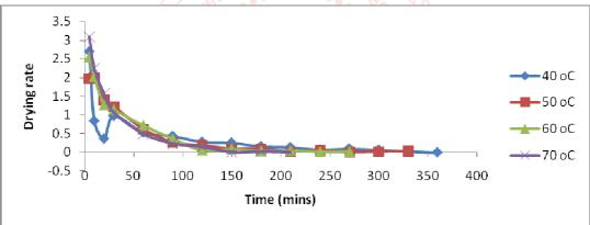
Fig. 17: Effect of temperature on drying rate of blanched aerial yam
