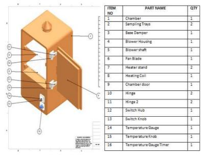
Fig 1: A Schematic diagram of convectional hot air dryer used
