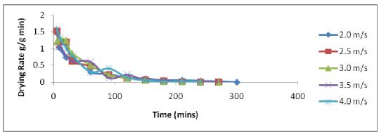
Fig. 15: Plot of drying rate of blanched aerial yam against time at different air speeds
