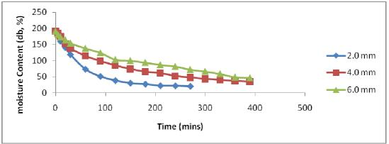
Figure 7: Effect of slice thickness on moisture content for drying of blanchedaerial yam.
