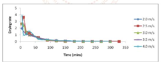
Fig. 14: Plot of drying rate of unblanched aerial yam against time at different air speeds
