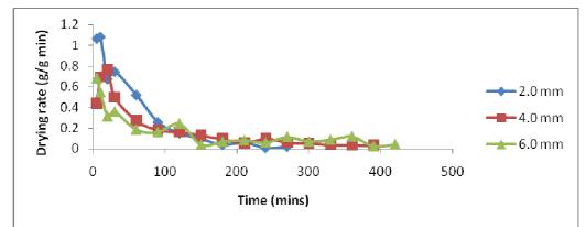
Fig. 12: Plot of drying rate against time at different slice thicknesses of unblanchedaerial yam.
