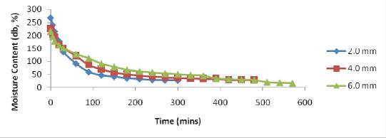
Figure 6: Effect of slice thickness on moisture content for drying of unblanchedaerial yam.
