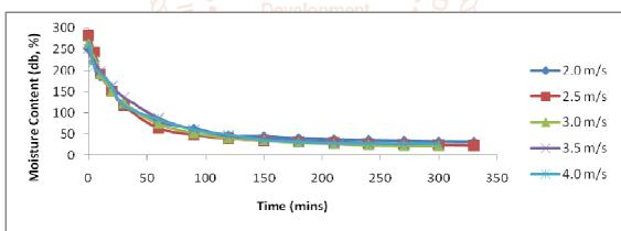
Fig. 8: Effect of drying air speed on moisture content of unblanched aerial yam.
