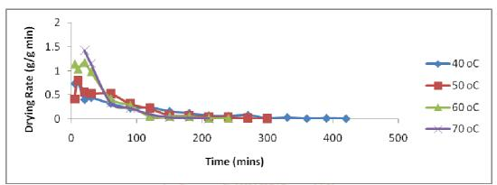
Fig. 16: Effect of temperature on drying rate of unblanchedaerial yam
