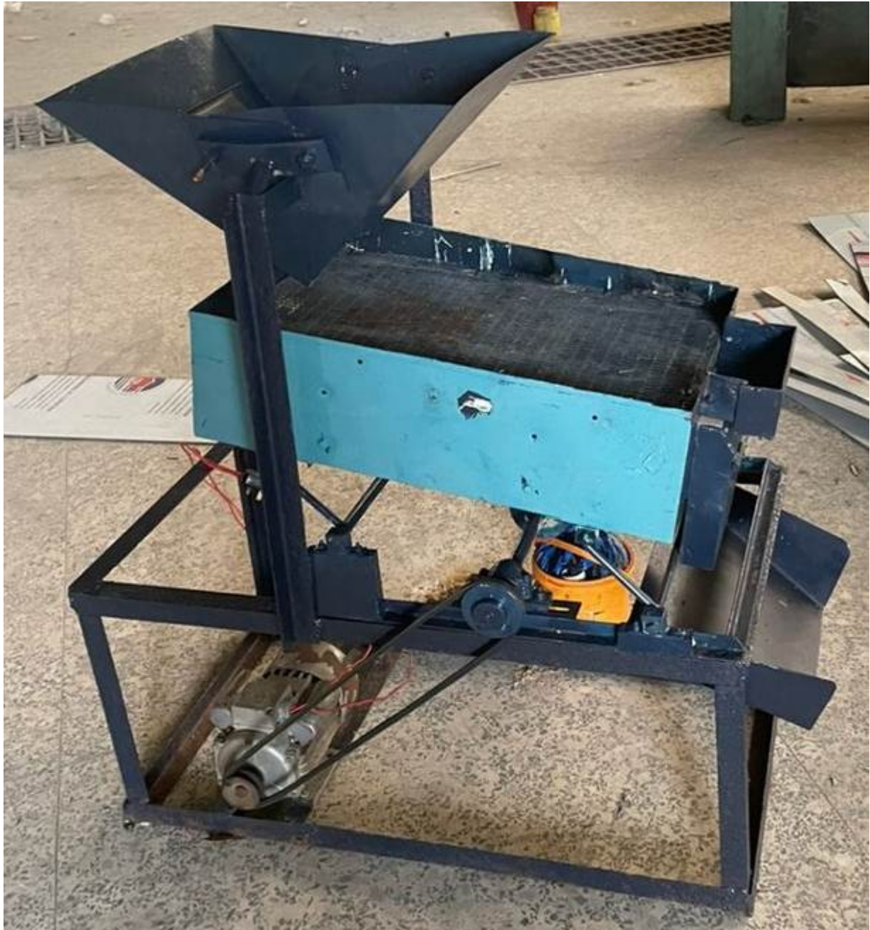
Figure 5: Fabricated Rice De-Stoning Machine
