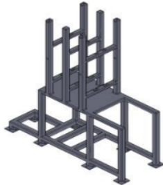
Fig. 2. UNP profile frame with bolt combination.
