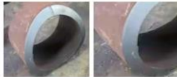
Figure 3.7 Cutting result with 46 mm gap
