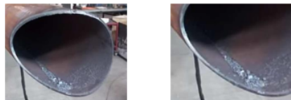
Figure 3.3 Cutting result with 42 mm gap
