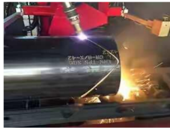
Figure 2.2 CNC pipe cutting process with torch
