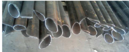
Figure 3.1 Cutting result with 30 mm gap
