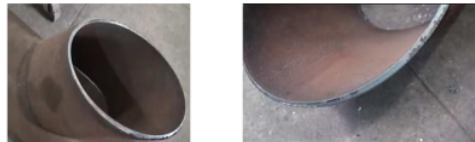
Figure 3.5 Cutting result with 44 mm gap
