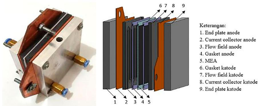
**Figure 1.** PEM fuel cell configuration.
