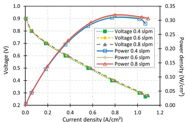
**Figure 5.** The effect of oxygen flow rate on current density and power density in the leaf-baffle flow field.
