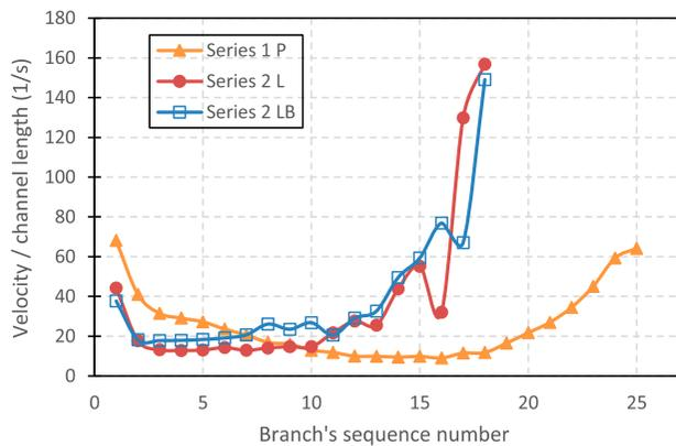
**Figure 7.** Comparison of branch entry velocity/channel length with flow field variations.
