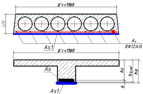
**Figure 2. Calculation scheme for strengthening the metal sheet from the lower part of the reinforced concrete plate by gluing it in a polymer solution.**
