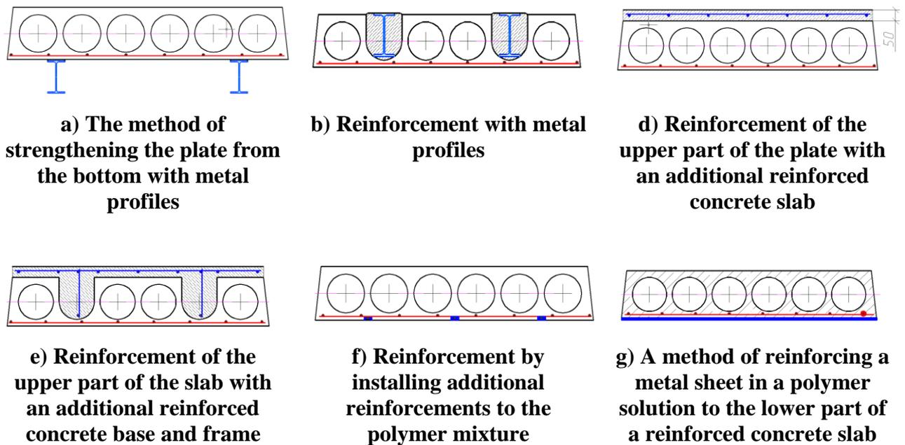
Figure 1. Methods of strengthening multi-cavity reinforced concrete slab.
