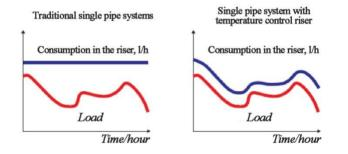
Figure 1. Schematic diagram of the operation of risers
