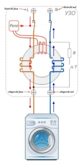
Figure 1. The principle of operation of the extinguishing protection equipment in the normal state
