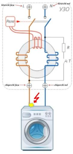
Figure 2. the principle of operation of the device in the event of a load loss
