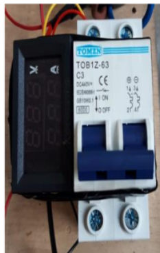
Fig. 7. DC MCB With Voltmeter And Amperemeters
