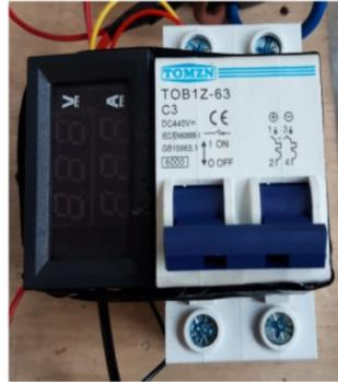
Figure 7. *DC MCB* With Voltage And Current Meters
