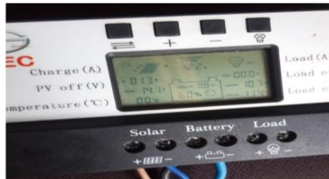
Figure 5. Solar Charge Controlled (SCC)
