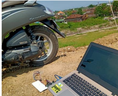
Figure 14. Accelerometer Testing at the Lapindo Embankment
