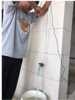
Figure 4. ultrasonic sensor testing in a water tank
