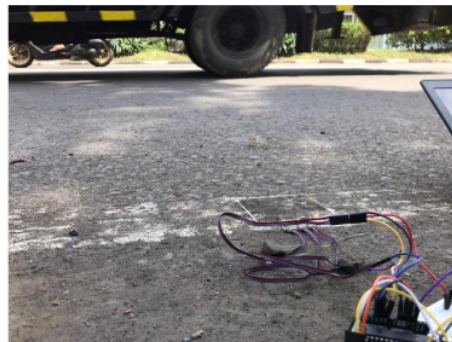
Figure 9. Accelerometer Sensor Testing on the Highway
