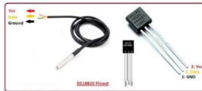
Gambar 1. Sensor suhu DS18B20[5]
