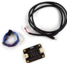
Gambar 2. Sensor TDS (Total Dissolve Solid) [8]
