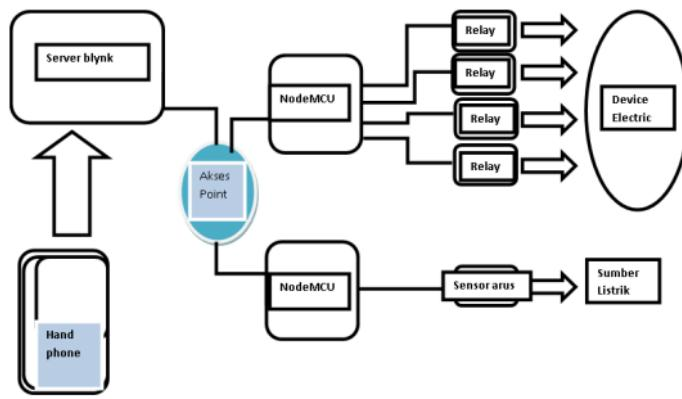
Figure 1. Blok diagram system
