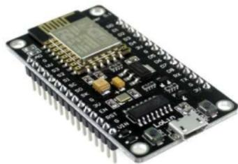
Gambar 1. NodeMcu ESP8266[5]
