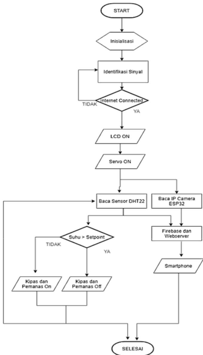
Gambar 4. Flowchart Sistem Monitoring
