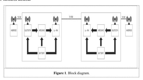
This is an overview of the tools used for short message media in the blank spot area. That is, an Android phone that is connected to a device that consists of Telemetry Lo Ra - Arduino Pro Mini — Bluetooth HC 05 and then connected to the battery (Figure 1).
